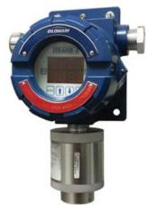
**Remote Diagnostics, Set-up or Calibration** The iTrans 2 fixed gas detector employs an intelligent electronics platform to provide one or two points of detection from a single head for maximum flexibility, superior performance and lower installation costs. With the optional HART Communication Protocol, the iTrans 2 offers remote diagnostics, set-up or calibration by superimposing a high-frequency current across the industry standard 4-20mA analog line.
